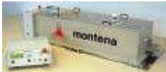
Marx pulse generator 350 kV, rise time 5 ns / duration 500 ns with control unit for Pulse Current Injection according to MIL STD 188/125, short pulse
